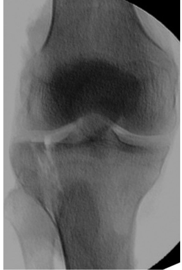
Figure 3. A fluoroscopy image taken after the axial loading-only test shows a tibial plateau fracture.
